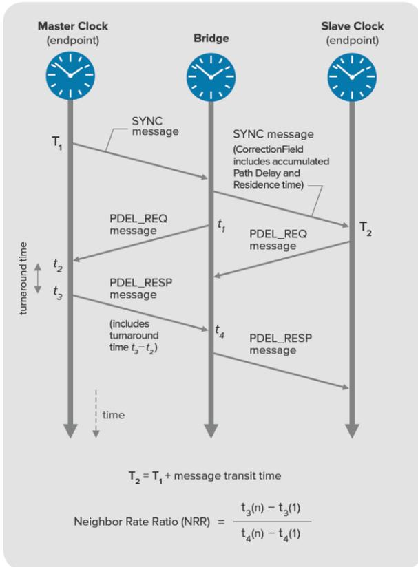
Peer Delay messages yield four timestamps (t1, t2, t3 and t4), from which it is possible to calculate the round-trip time for messages from the initiator to responder, and back, and ultimately the path delay.
