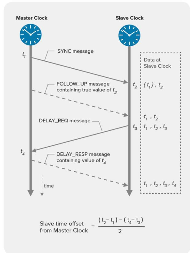
These messages yield four timestamps ( $t_1$ ,  $t_2$ ,  $t_3$  and  $t_4$ ), from which it is possible to calculate the round trip time for messages from the master to the slave, and back to the master (assuming that the slave clock is advancing at a similar rate to the master).
