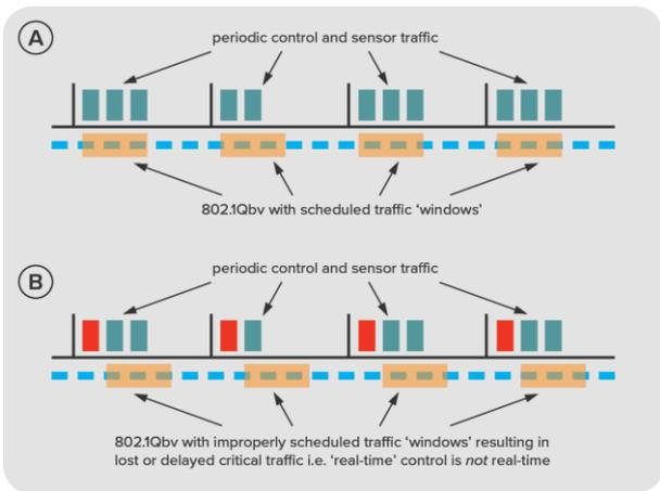
As a result, timing calculations have run using incorrect timing information, ultimately causing traffic to be incorrectly delayed and dropped. In the case of critical command messages in a deployed system, this could result in mistiming and damage to machinery, incurring costly downtime.
